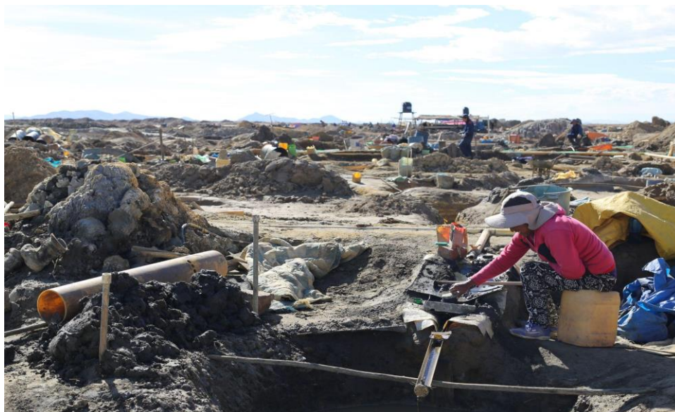
Figure 13: Miners leaching tin from waste rock using buddle pits directly on the soil with no further protection, in Machacamarca (Oruro, Bolivia). © Isabella Szukits (Südwind)
