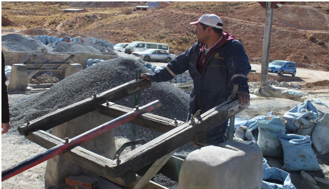
Figure 12: Miner separating zinc-silver and lead-silver minerals by gravity before their concentration, at Cooperativa Minera San José Jallpa Socavón (Oruro, Bolivia). © Silke Ronsse (CATAPA)
