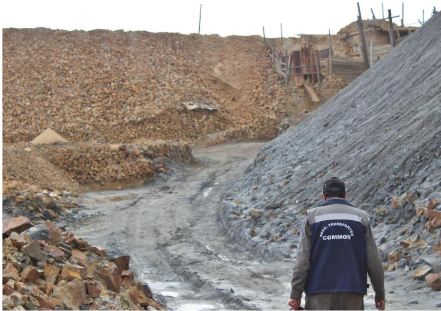
Figure 14: Heaps of waste rock (without any environmental measure applied) from different minerals at Cooperativa Minera Morococala (Oruro, Bolivia). © Silke Ronsse (CATAPA)
