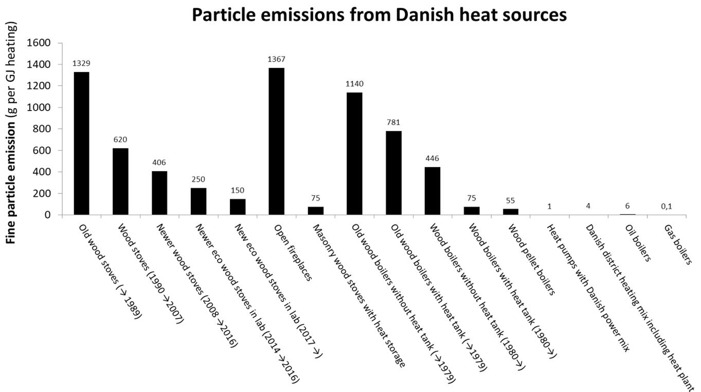
Figure 1 shows that new wood stoves/boilers—under optimal laboratory conditions—emit less particulate matter (PM<sub>2.5</sub>) than older appliances. However, the figure also shows that emissions from other heat sources (heat pumps, district heating, oil boilers and gas boilers) are much lower than even the newest and most efficient wood stoves/boilers operating under optimal conditions (dry firewood, perfect chimney draught as well as optimal user management). Replacing old
