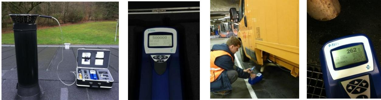
The pictures show that the concentration of ultrafine particles in the wood smoke is above the detection limit of the device (500,000 particles per cm<sup>3</sup>), even during optimal conditions in an ecolabel stove with no visible smoke from the chimney. For comparison, the concentration in the exhaust of a truck with particulate filter is about 250 i.e., at least 2,000 times less.
